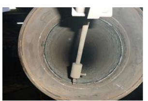
← the leading torch angle and torch position relative to the bottom of the pipe.
